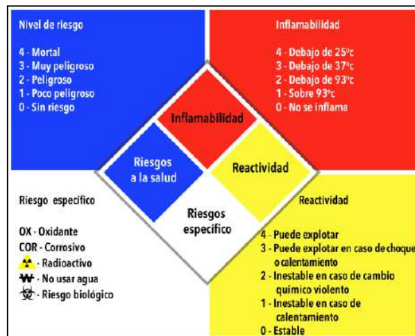
Imagen 12. Rombo NFPA (National Fire Protection Association).
